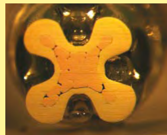
Crimp-cross section HARTING crimp profile
